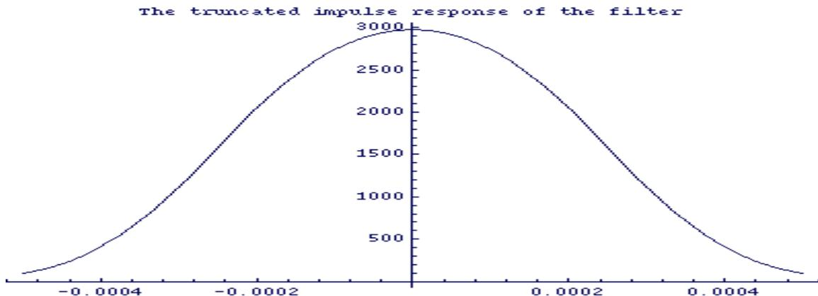
**Fig 2. The Turnonated Impulse response of the filter**
