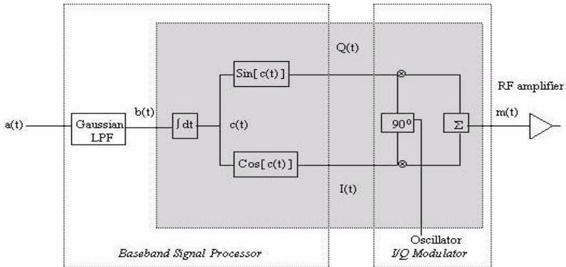
**Fig 1. GMSK implemented by quadrature baseband method**
