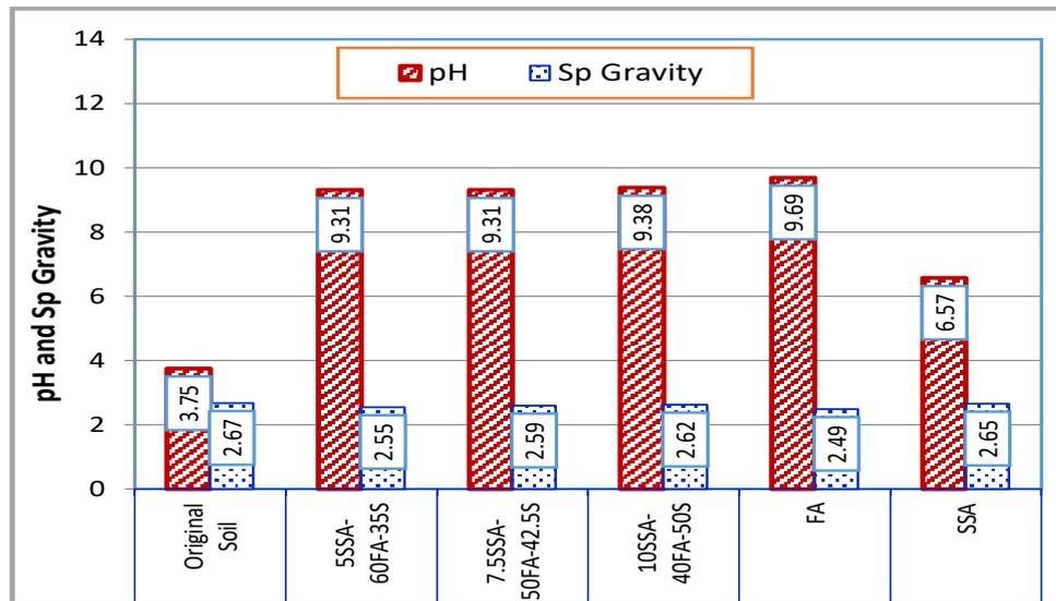
Figure 4: Variations of pH and Specific Gravity with SSA-FA Content
