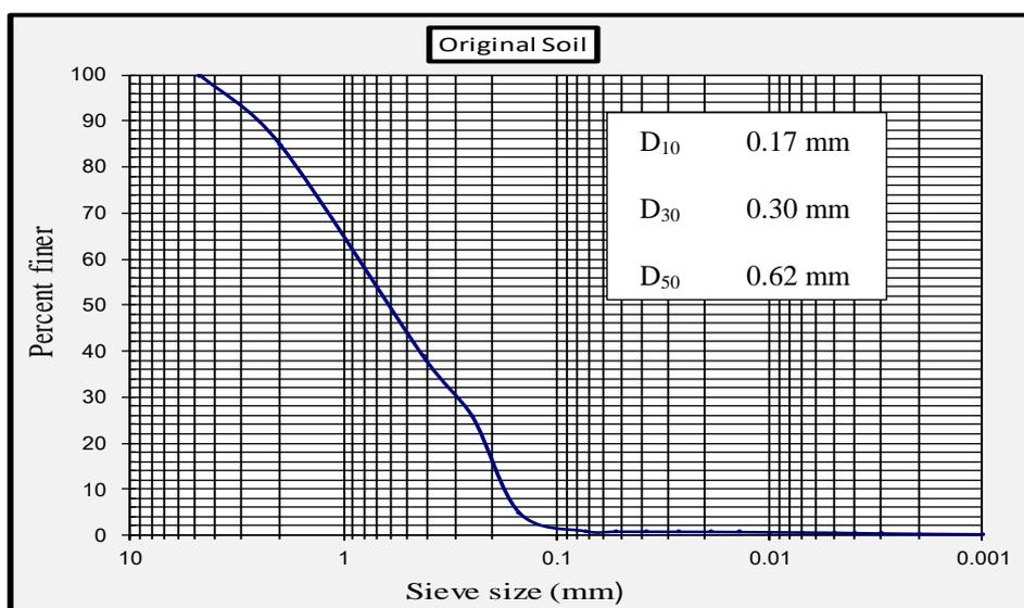
Figure 3: The Grain Size Distribution Curve for The Soil Used in The Study
