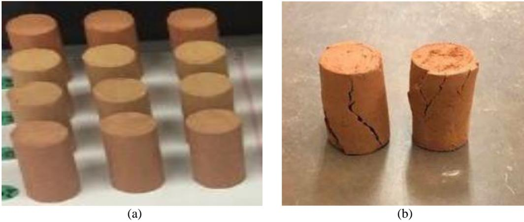
**Figure 6: Appearance Typical Test Specimens (a) Before (b) After The UCS Test**
