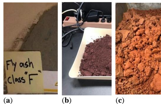
**Figure 1: A Typical Appearance of (a) Class F FA (b) SSA, and (c) Soil Used in This Study**
