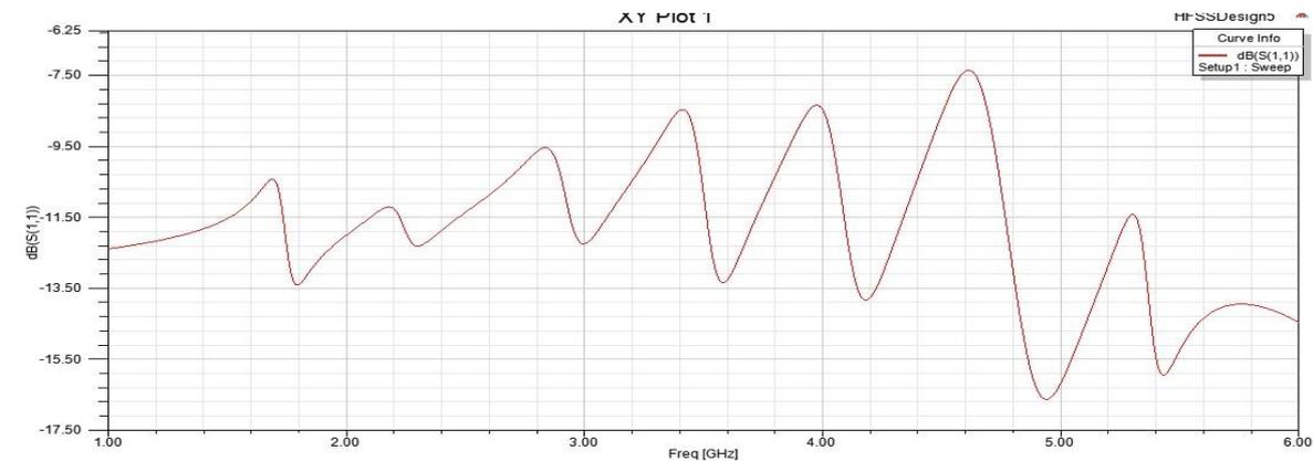
**Figure 4: S11Vs Frequency Curve for First Iterative Antenna**
