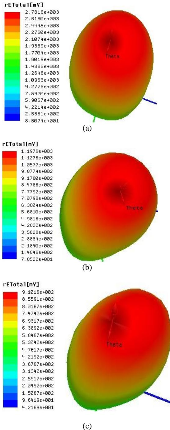
**Figure 5: 3-D Radiation Pattern of Design Fractal Antenna**
