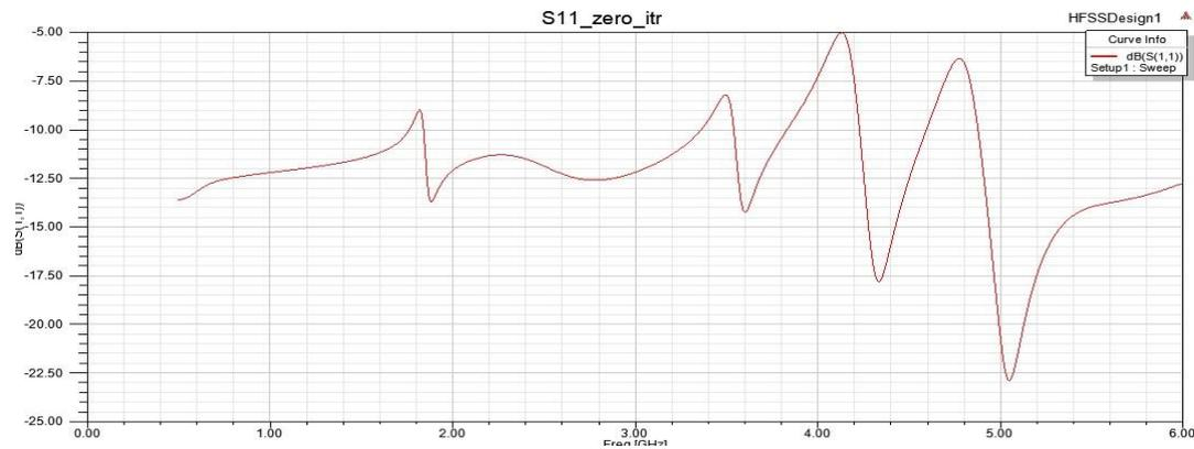
**Figure 2: S11Vs Frequency Curve for Base Antenna**
