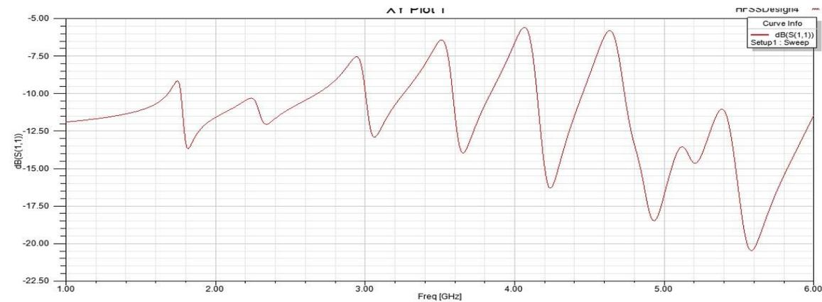
**Figure 3: S11Vs Frequency Curve for First Iterative Antenna**
