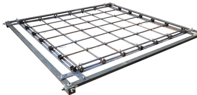
Figure 5: The Developed Mat Bar Setter with Steel Bars
