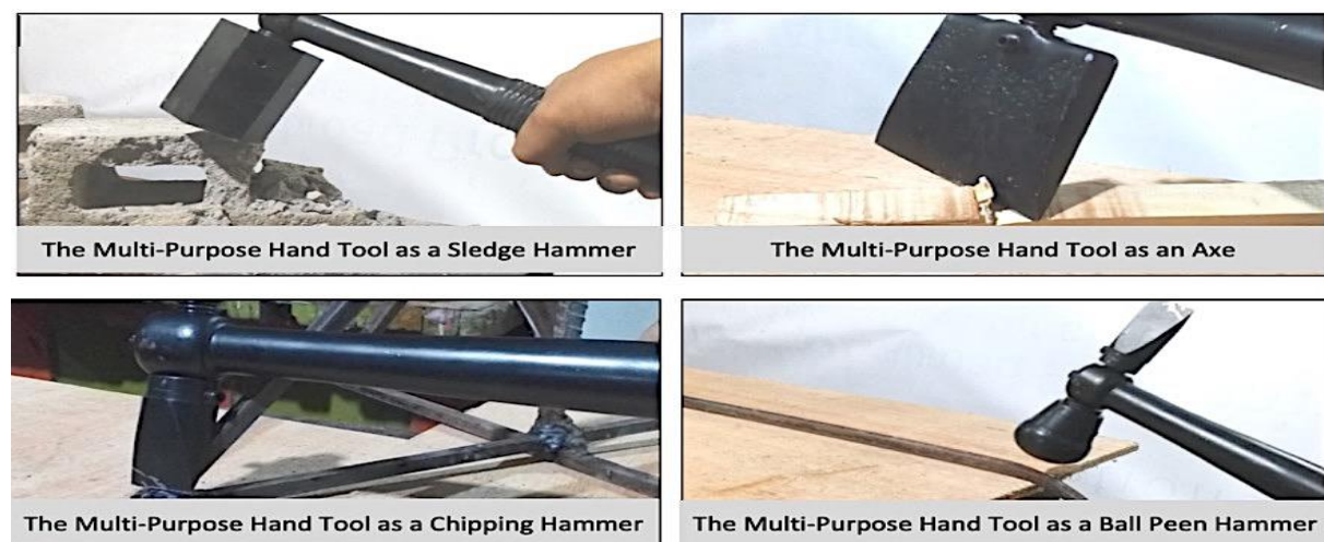
Figure 6: The Hand Tool As Sledge Hammer, Axe, Chipping Hammer and Ball Peen Hammer
