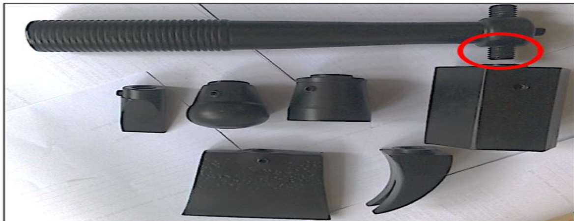
Figure 4: The Handle and Attachments of The Multi-Purpose Hand Tool with Threading
